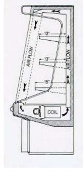
See SHELVES for the special loading instructions. Air flows out of the honeycomb diffuser located above the product, across the product, and into the return duct. The honeycomb can be removed for cleaning.
