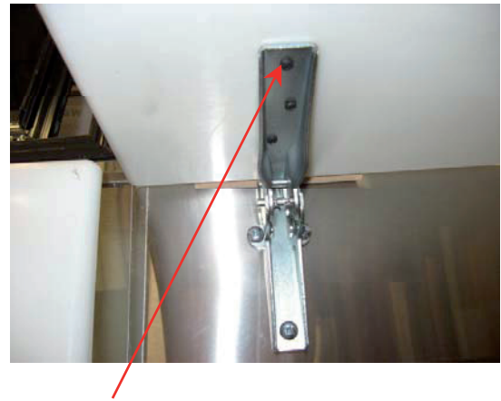
Step 8: screw bracket into wrap board (screws provided -#8 X 1 1/4")
