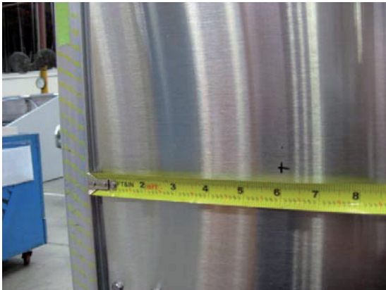
Step 1: Measure 6 inches from wrapping board end.
