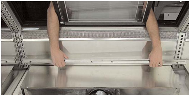
STEP 6 – Lift out display pan support.
