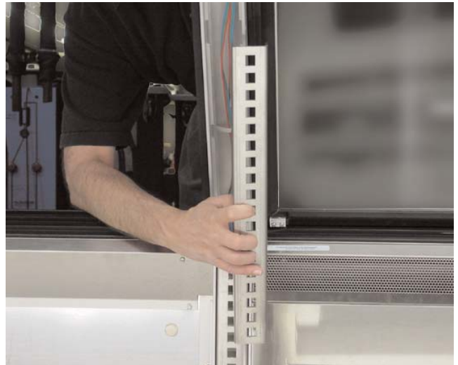
STEP 9 – Lift out upper shelf supports.
