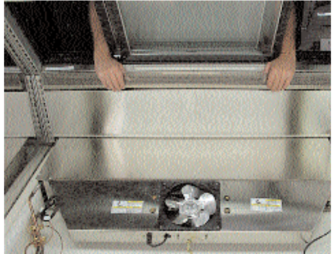
STEP 9 – Lift out upper shelf supports.
