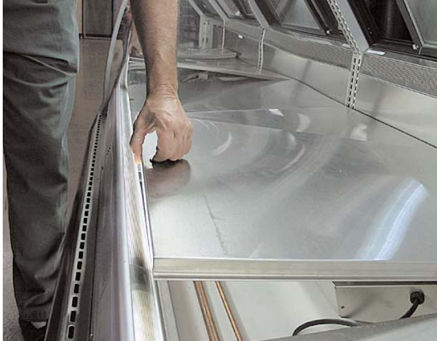
STEP 6 – Lift out display pan support.
