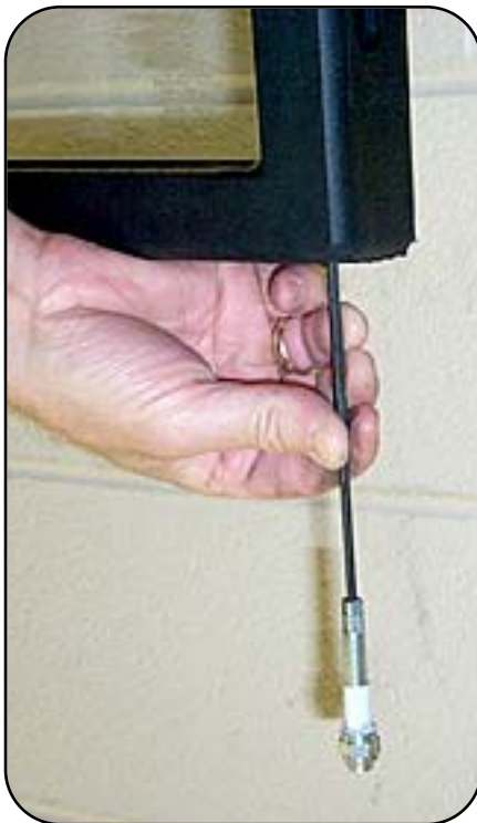
Figure 8. Replacing Door Hinge Spring Assembly
